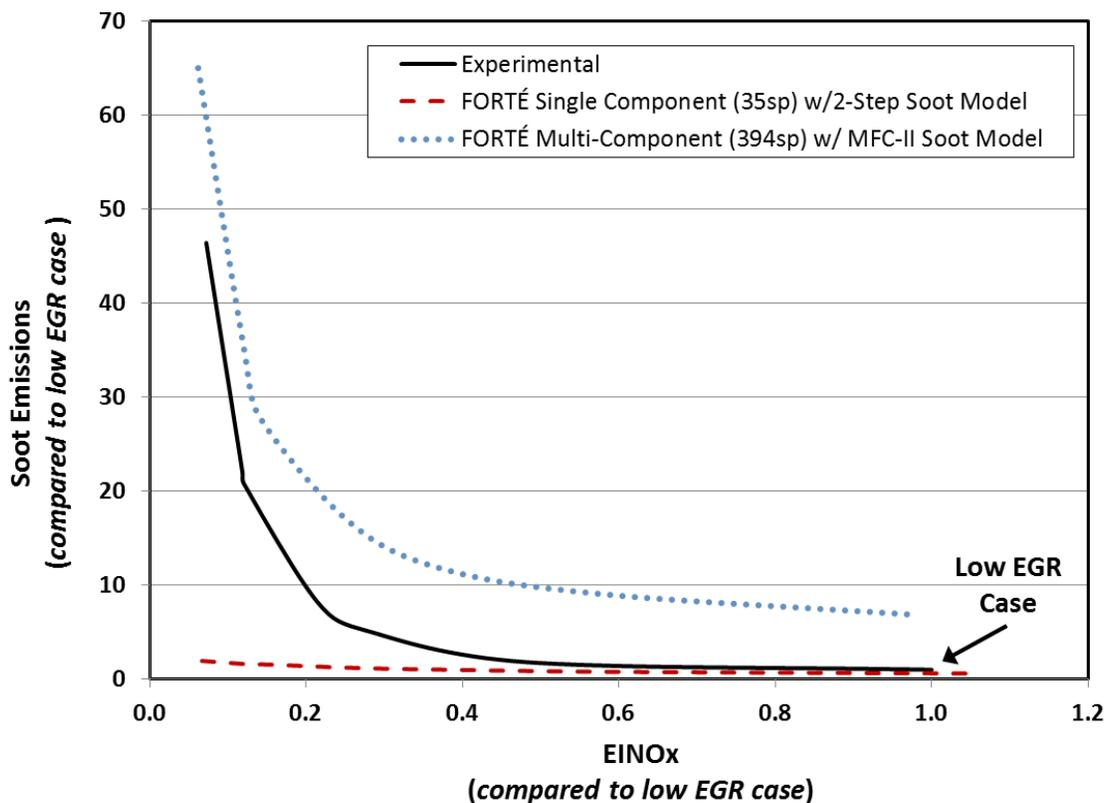
Figure 2. Comparison of FORTÉ soot and NO<sub>x</sub> results in a high EGR diesel simulation using multi-component MFC soot model and traditional 2-step soot modeling approach.
