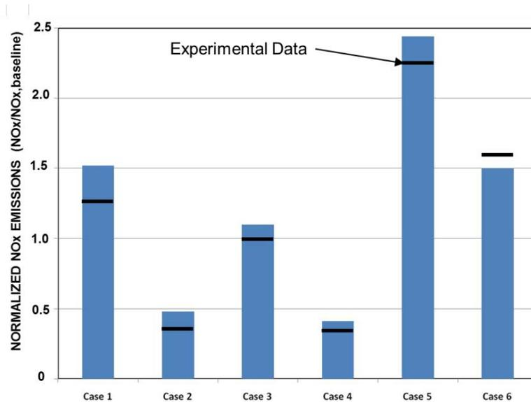
Figure 3. ENERGICO NO<sub>x</sub> emissions results capture impacts of variable fuel composition.
