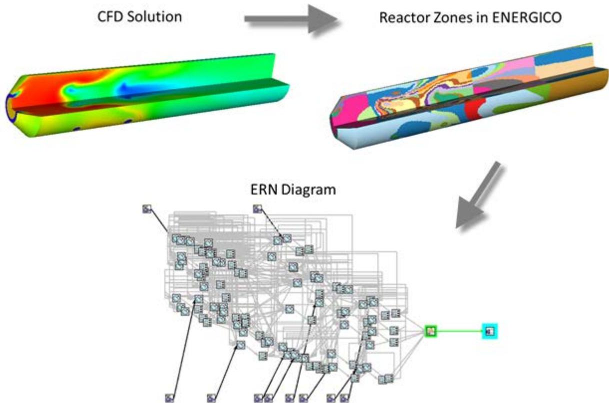
Figure 1. ENERGICO workflow starting from a CFD solution, dividing the chemical process into Zones that become reactors in the ERN.
