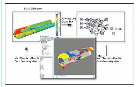
The ENERGICO software package from Reaction Design is used to solve complex combustion challenges in gas turbines by virtual simulation. It automatically creates and solves Equivalent Reactor Networks (ERN) from CFD analysis programs. Viewing the ERN results on combustor geometry facilitates the design modifications.
